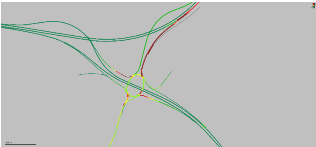
Figure 4.22: A12 J29 PM peak 2043 VISSIM new local plan without mitigation heatmap
