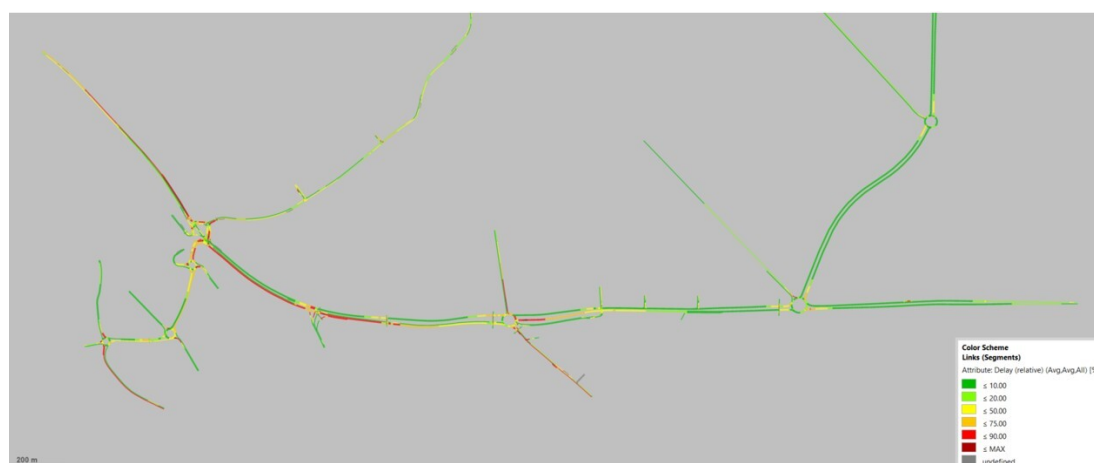
Figure 4.31: A133 Clingoe Hill AM peak 2043 VISSIM new local plan with mitigation heatmap
