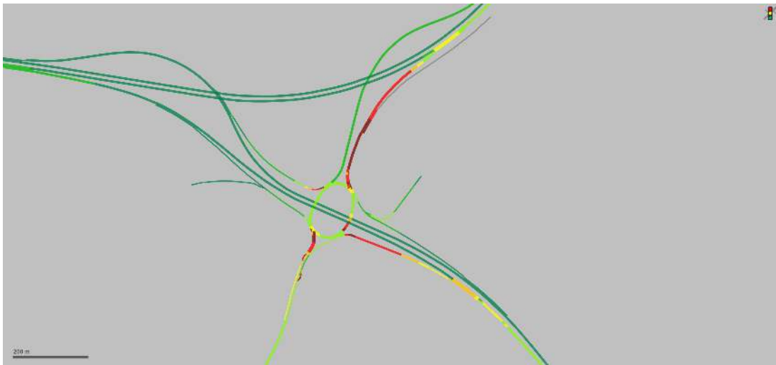
Figure 4.21: A12 J29 AM peak 2043 VISSIM new local plan without mitigation heatmap
