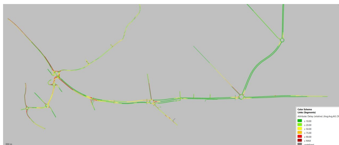
Figure 4.32: A133 Clingoe Hill PM peak 2043 VISSIM new local plan with mitigation heatmap
