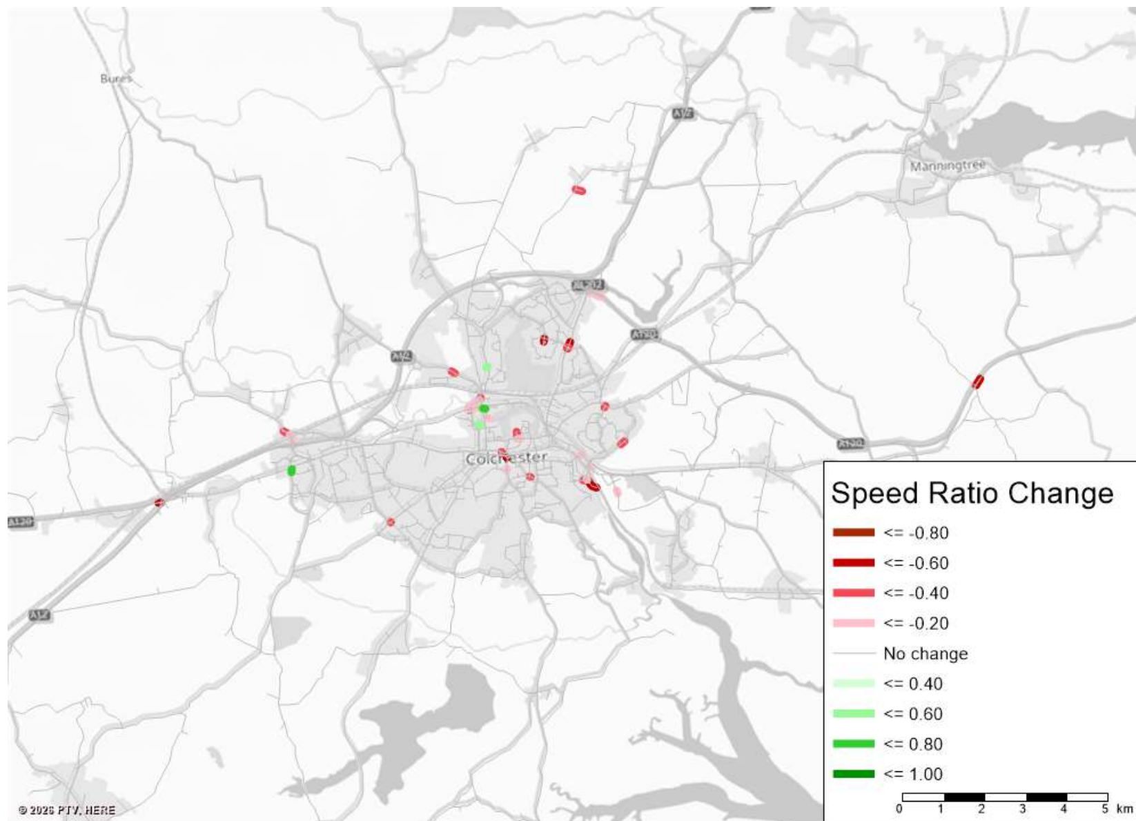
Figure I.14: PM Difference in traffic speed between Scenario 6 and Scenario 5
