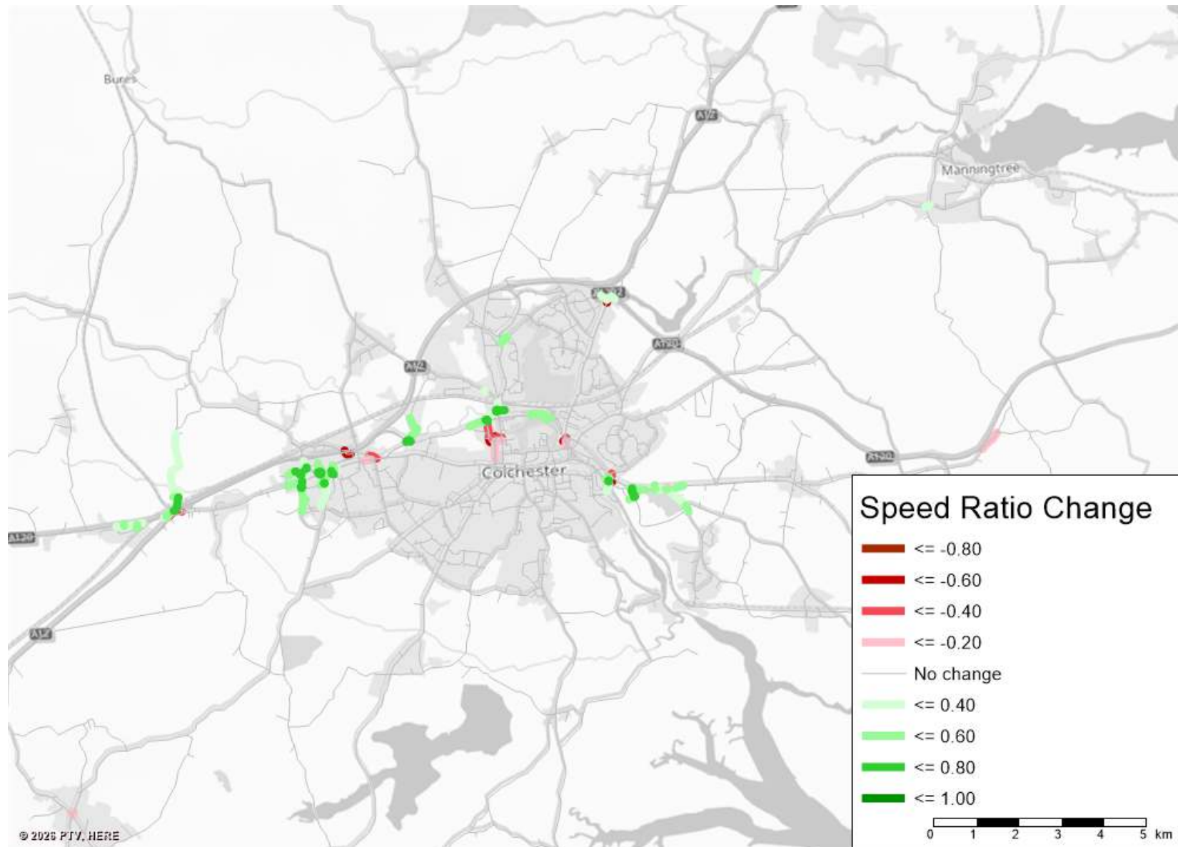
Figure 4.1: AM Difference in traffic speed between Scenario 3 and Scenario 2
